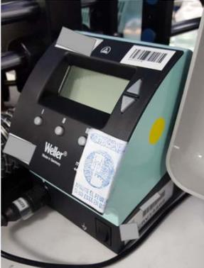
A photograph of a Weller soldering station, a device used for heating and applying solder to electronic components. It has a digital display and a barcode label on the front panel.                                                           | <p>Cod: 14489<br/>Activo: 40210W<br/>Ubicación: Incorrecta</p> |
