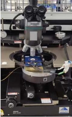
A photograph of a Hawkeye Alessi Probe Station, a precision instrument used for measuring the electrical properties of microelectronic components. It features a central probe head with multiple contact points, mounted on a rotating stage. | <p>Cod: 11455<br/>Activo: 11041P<br/>Ubicación: Correcta</p>   |
